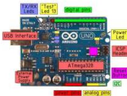
Gambar 6. Board Arduino Uno
