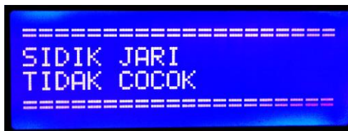
Figure 8. LCD Display When Fingerprint Input Is Not Matching
