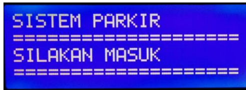
Figure 7. LCD Display When Fingerprint Input Is Matching With Database
