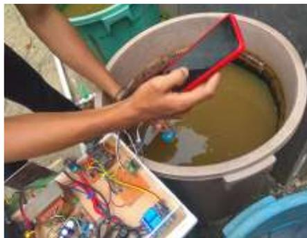
Gambar 9. Pengujian sensor turbidity
