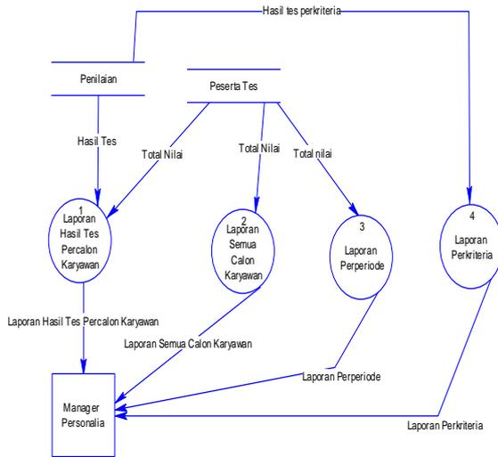
**Gambar 3. Diagram Alir Data Level 1 Proses 3 SPK**
